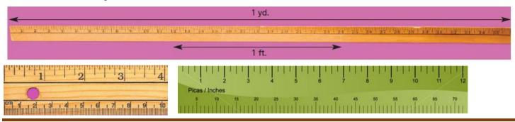
To measure the length of an object, you must first determine the smallest indicated unit by counting the number of divisions between two adjacent inch marks. The ruler below has 16 divisions between two adjacent inch marks, so the smallest indicated unit is  $\frac{1}{16}$  of an inch, which is written as  $\frac{1}{16}$  in.
